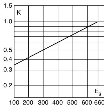
For other power factor values, the total clearing integral can be calculated as a multiple of the clearing integrals, the correction factor K and the correction factor X.
