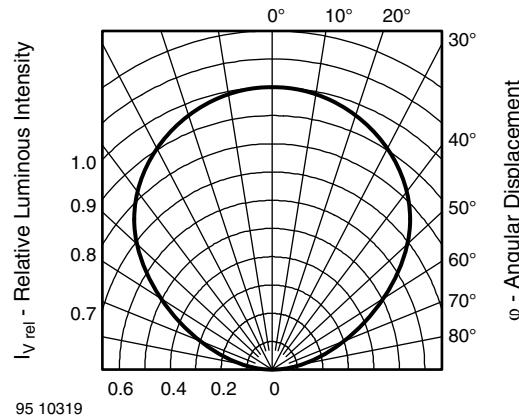
Fig. 11 - Relative Luminous Intensity vs. Angular Displacement
