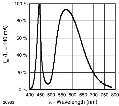
Fig. 9 - Relative Spectral Emission for Natural White
