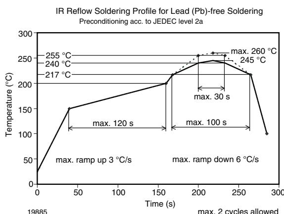
Fig. 12 - Vishay Lead (Pb)-free Reflow Soldering Profile
