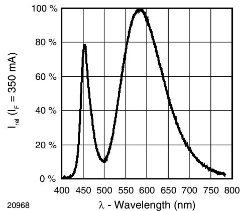
Fig. 10 - Relative Spectral Emission for Warm White
