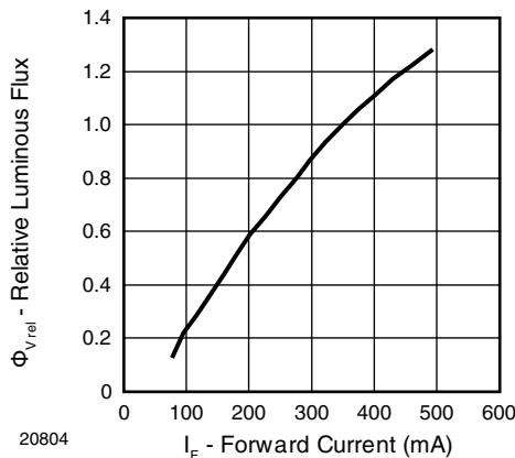
Fig. 1 - Relative Luminous Flux vs. Forward Current
