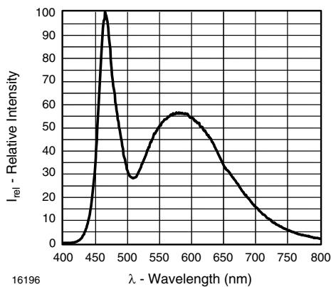
Fig. 8 - Relative Spectral Emission for Cool White
