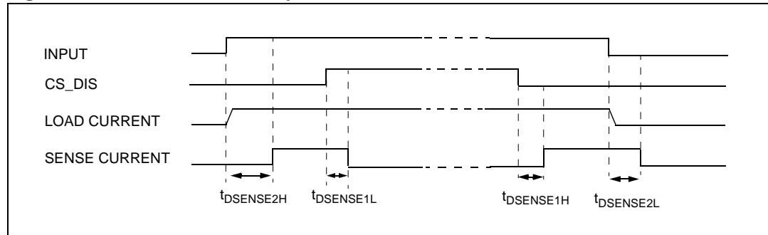
**Figure 5. Open load Off-state delay timing**
