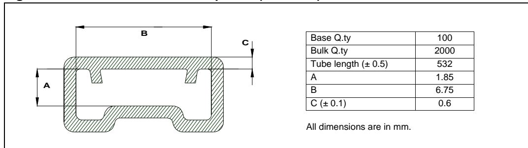
**Figure 41. PowerSSO-12 tape and reel shipment (suffix "TR")**
