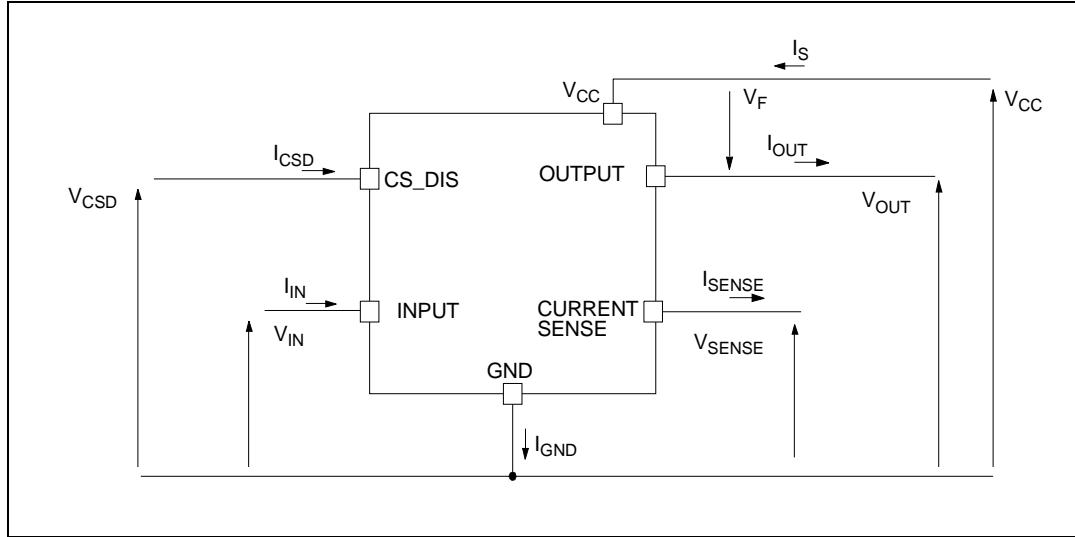
Note:  $V_F = V_{OUT} - V_{CC}$  during reverse battery condition.
