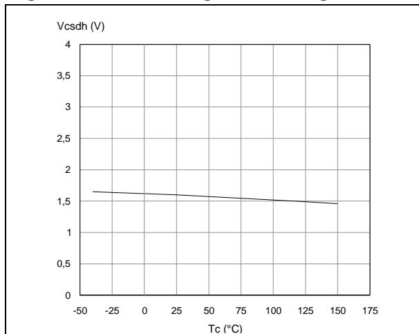
**Figure 30. CS\_DIS clamp voltage**
