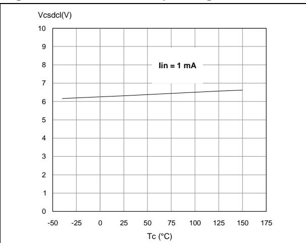
**Figure 31. CS\_DIS low level voltage**
