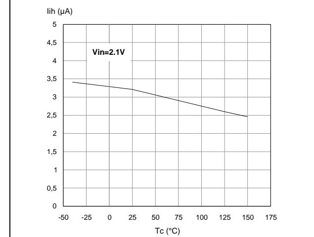
**Figure 19. Input clamp level**
