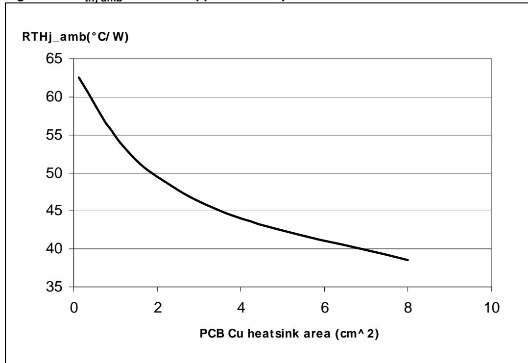
Figure 37. PowerSSO-12 thermal impedance junction ambient single pulse
