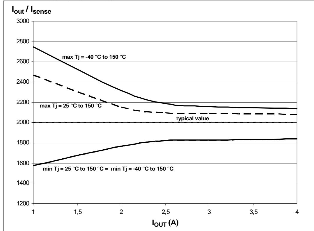
**Figure 10.** Maximum current sense ratio drift vs. load current
