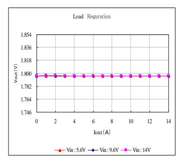
Fig. 12-3-7. Output Voltage v.s. Output Current
