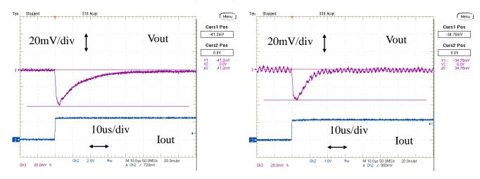
Fig. 12-1a. Load Transient Response (MPDRX301S)
