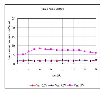
Fig. 12-3-12. Ripple Voltage v.s. Output Current
