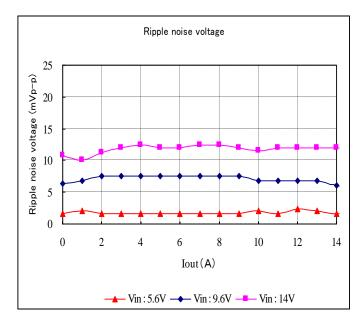
Fig. 12-3-18. Ripple Voltage v.s. Output Current
