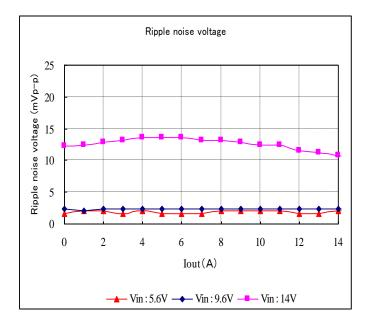
Fig. 12-3-6. Ripple Voltage v.s. Output Current
