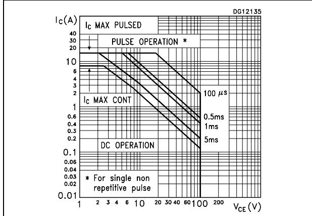
**Figure 3. Derating curve**
