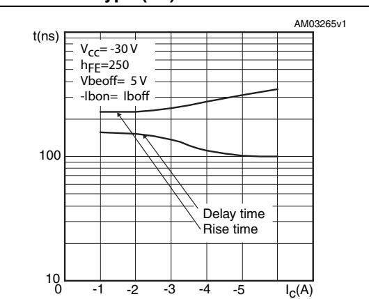
**Figure 14. Resistive load switching times for NPN type (off)**
