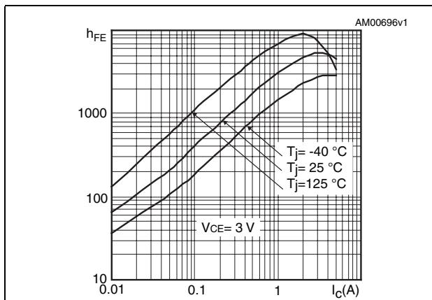
**Figure 5. DC current gain for PNP type**
