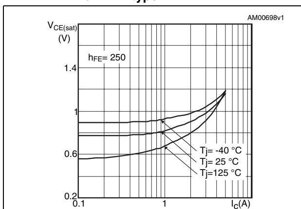
**Figure 7. Collector-emitter saturation voltage for PNP type**
