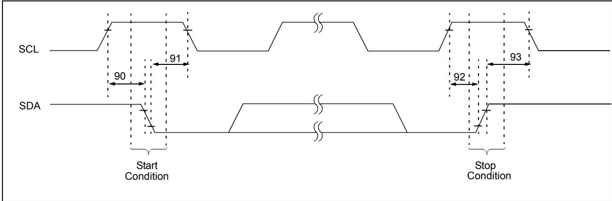
**TABLE 28-20: MASTER SSP I<sup>2</sup>C™ BUS START/STOP BITS REQUIREMENTS**
