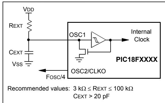
The RCIO Oscillator mode (Figure 3-6) functions like the RC mode, except that the OSC2 pin becomes an additional general purpose I/O pin. The I/O pin becomes bit 6 of PORTA (RA6).
