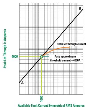
Figure 19 – Determining Threshold Current from Peak
