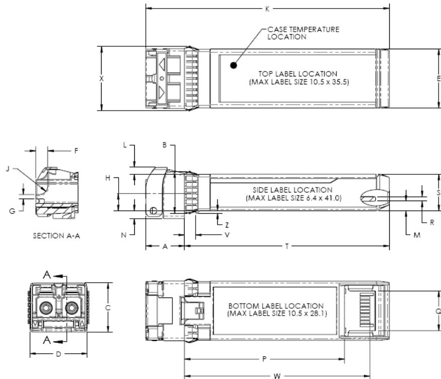
Figure 2. Mechanical Dimensions
