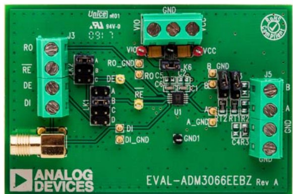
Figure 1. EVAL-ADM3066EEBZ Evaluation Board
