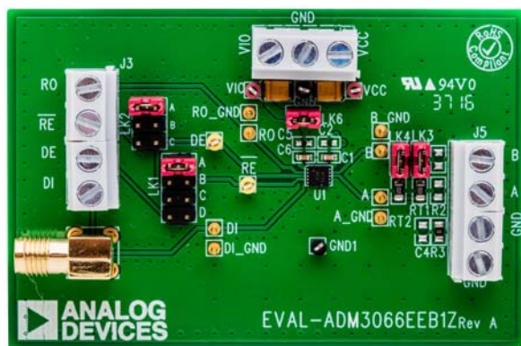
Figure 2. EVAL-ADM3066EEB1Z Evaluation Board
