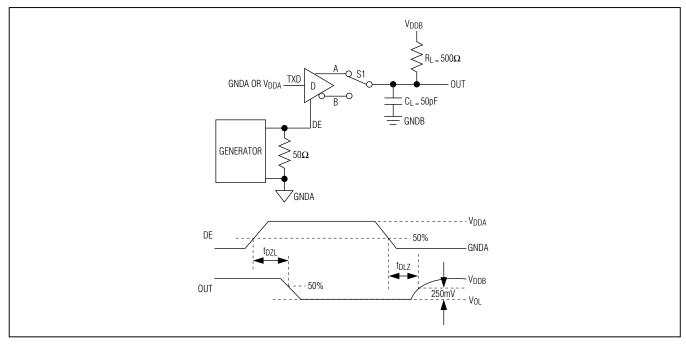
Figure 6. Driver Enable and Disable Times ( $t_{DZL}$ ,  $t_{DLZ}$ )
