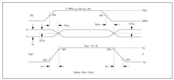
Figure 4. Driver Propagation Delays
