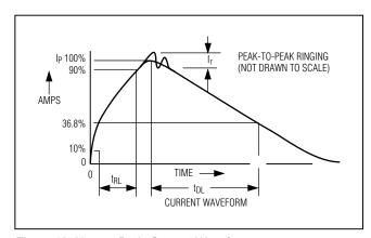
Figure 13. Human Body Current Waveform
