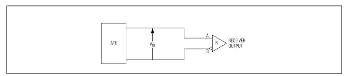
Figure 7. Receiver Propagation Delay Test Circuit
