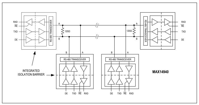
Figure 10. Typical Isolated Half-Duplex RS-485 Application
