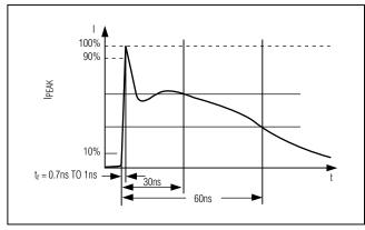
Figure 14. IEC 61000-4-2 ESD Test Model
