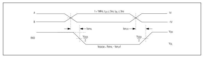
Figure 8. Receiver Propagation Delays
