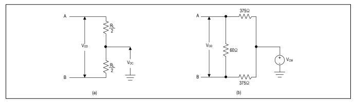
Figure 1. Driver DC Test Load
