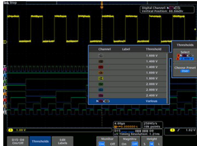
With color-coded digital waveform display, groups are created by simply placing digital channels together on the screen, allowing digital channels to be moved as a group.
