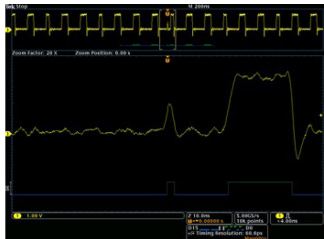
The MagniVu high-resolution record provides 60.6 ps timing resolution, enabling you to take critical timing measurements on your digital waveforms.
