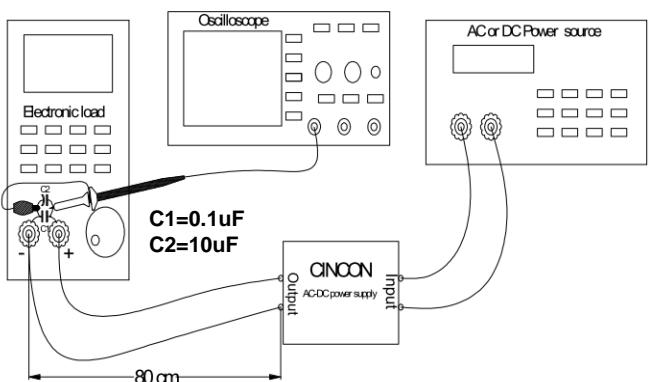
Figure 2. Output Voltage Ripple and Noise Measurement
