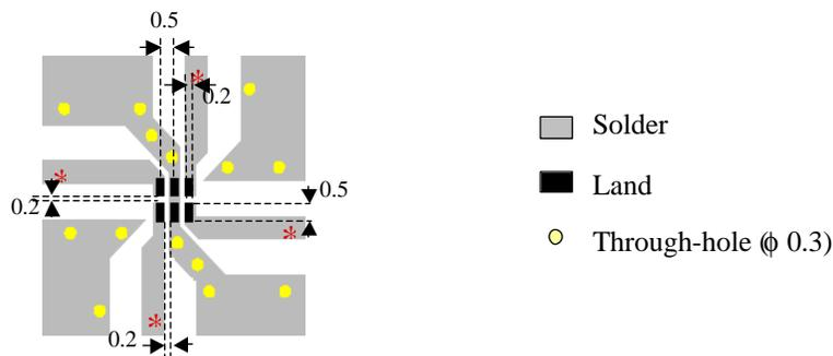
\* Line width should be designed to match 50ohm characteristic impedance, depending on PCB material and thickness.
