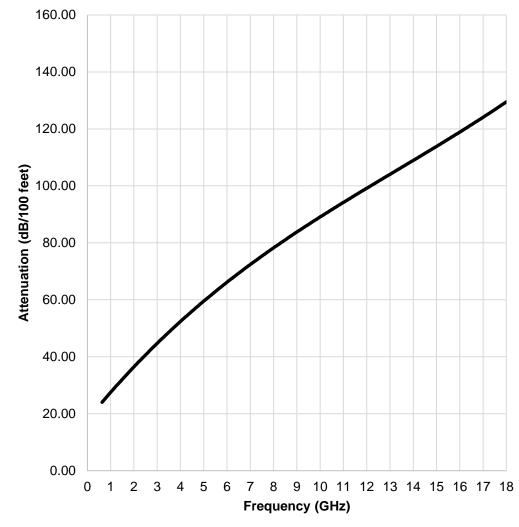
CHECKED GENERAL TOLERANCE CREATED Würth Elektronik eiSos GmbH & Co. KG EMC & Inductive Solutions JaC DaSc DIN ISO 2768-1m Max-Eyth-Str. 1 74638 Waldenburg **SMA Straight Plug to SMA Straight** Tel. +49 (0) 79 42 945 - 0 **Bulkhead Jack on Hand-Formable** ORDER CODE www.we-online.com 65503503215308 Cable .085 WR-CXASY eiSos@we-online.com DATE (YYYY-MM-DD) BUSINESS UNIT PAGE 001.001 Valid 2018-05-24 3/5 **WÜRTH ELEKTRONİK**
