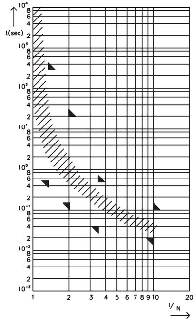
FI = 1.43 (max. operating current:  $0.7 \times I_{\text{rat}}$  at 23°C)
