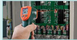
Detect hot spots on circuit breaker panels
