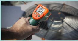
Test for temperature in HVAC systems
