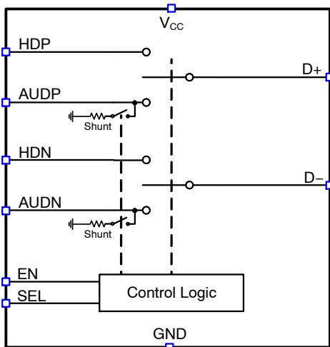
Figure 1. Block Diagram
