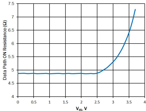
**Figure 14. Data Path On Resistance**
