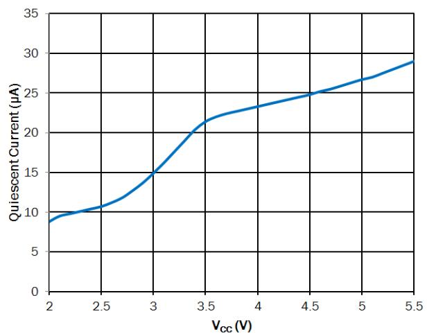
**Figure 13. Product Supply Current**
