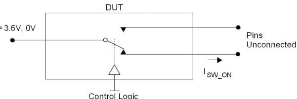
**Figure 9. On State Leakage**
