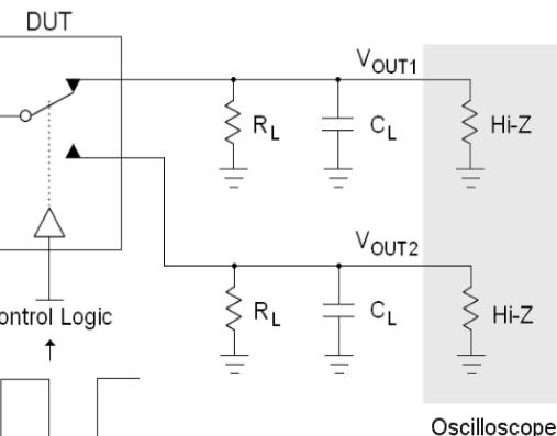
**Figure 7.  $t_{ON}$  and  $t_{OFF}$**
