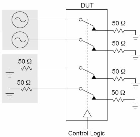
**Figure 5. Differential Crosstalk ( $S_{DD21}$ )**
