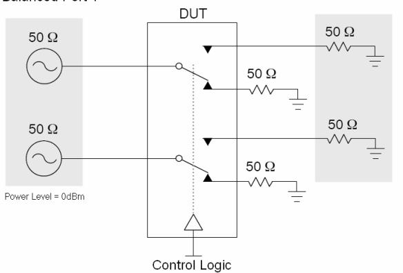
**Figure 4. Differential Off Isolation ( $S_{DD21}$ )**
