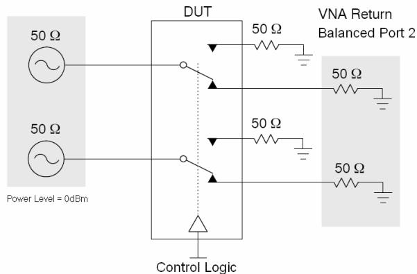
**Figure 3. Differential Insertion Loss ( $S_{DD21}$ )**
