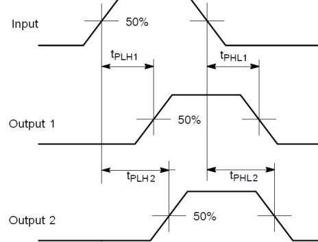
**Figure 6. Bit-to-Bit and Channel-to-Channel Skew**
