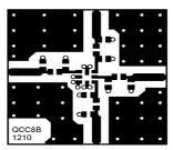
Optimised PCB layout for SAW filters in QCC8G package, pinning 1 - 5,6,7 (top side, scale 1:1)
