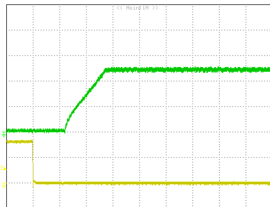
Figure 19: Turn on delay time at remote on 12Vin, 2.5V/30A out. (Green: VOUT, 1V/div, Yellow: ON/OFF, 2V/div, 1mS/div)
