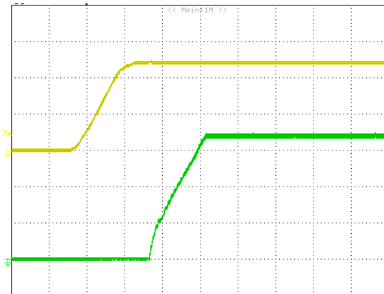
Figure 13: Turn on delay time at 12Vin, 1.8V/30A out. (Green : VOUT, 0.5V/div, Yellow: VIN, 5V/div. 1mS/div)
