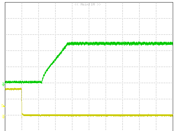
Figure 19: Turn on delay time at remote on 12Vin, 2.5V/30A out. (Green: VOUT, 1V/div, Yellow: ON/OFF, 2V/div, 1mS/div)
