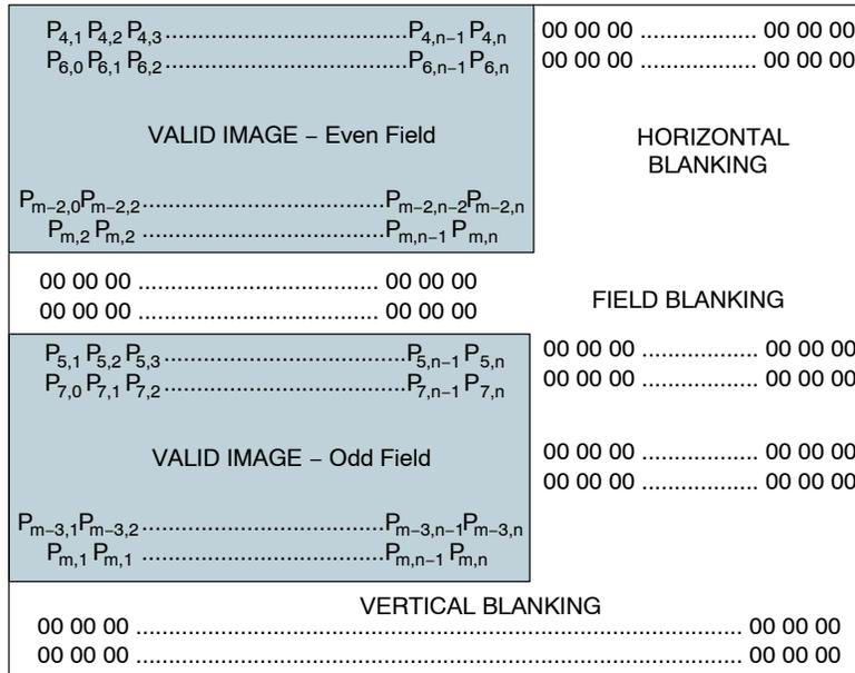
**Figure 33. Spatial Illustration of Interlaced Image Readout**
