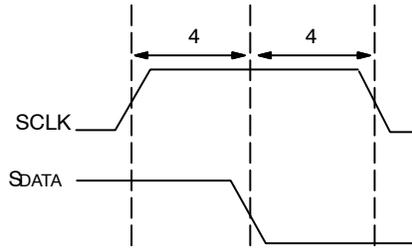
**Figure 40. Serial Host Interface Start Condition Timing**
