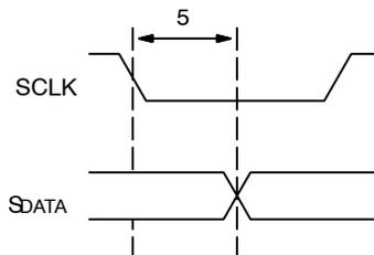
Note: SDATA is pulled LOW by the sensor, or allowed to be pulled HIGH by a pull-up resistor off-chip.
