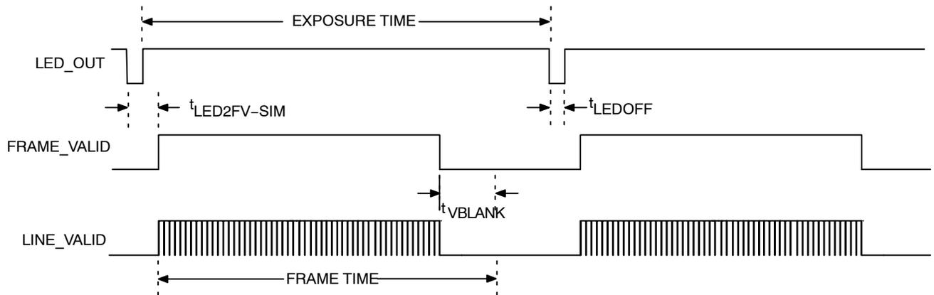
Figure 14. Simultaneous Master Mode Synchronization Waveforms #2
