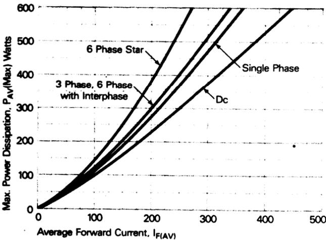
Figure 3. Power dissipation vs. Average forward current.
