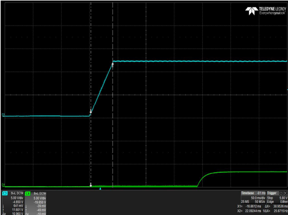
Figure 7: DS1600SPE-3 Output Voltage Startup – Vin = 90Vac Full Load: I_o = 63.2A , I_{sb} = 3.5A Ch 3: Vo Ch 4: Pwr_Good
