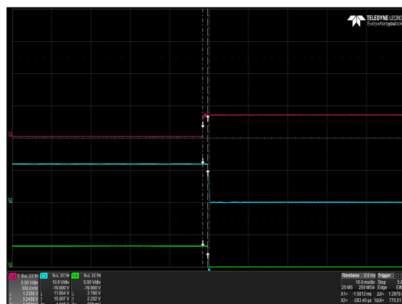
Figure 12: DS1600SPE-3 Turn Off Characteristic via PS_KILL_L Full Load: I_o = 129.8\text{A} , I_{sb} = 3.5\text{A} Ch 2: PS_KILL_L Ch 3: Vo Ch 4: Pwr_Good
