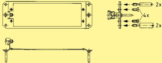
Retaining frame with 2 contact sockets and ground termination
