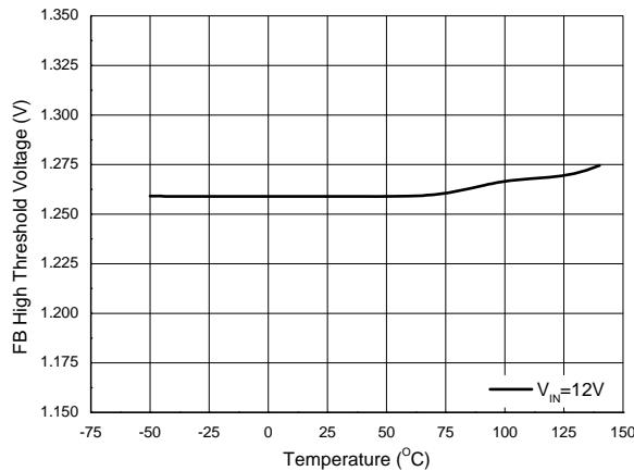
Figure 16. FB High Threshold Voltage vs. Temperature
