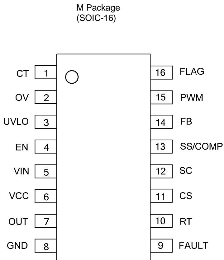
Figure 2. Pin Configuration of AP3041 (Top View)
