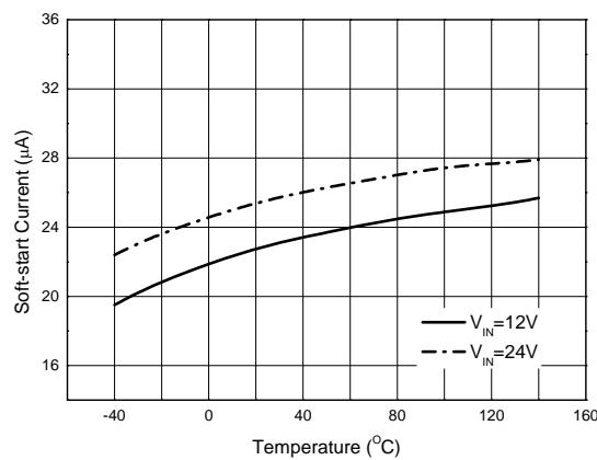
Figure 18. Soft-start Current vs. Temperature
