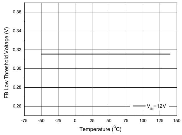
Figure 15. FB Low Threshold Voltage vs. Temperature
