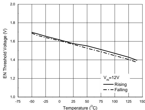
Figure 12. EN Threshold Voltage vs. Temperature
