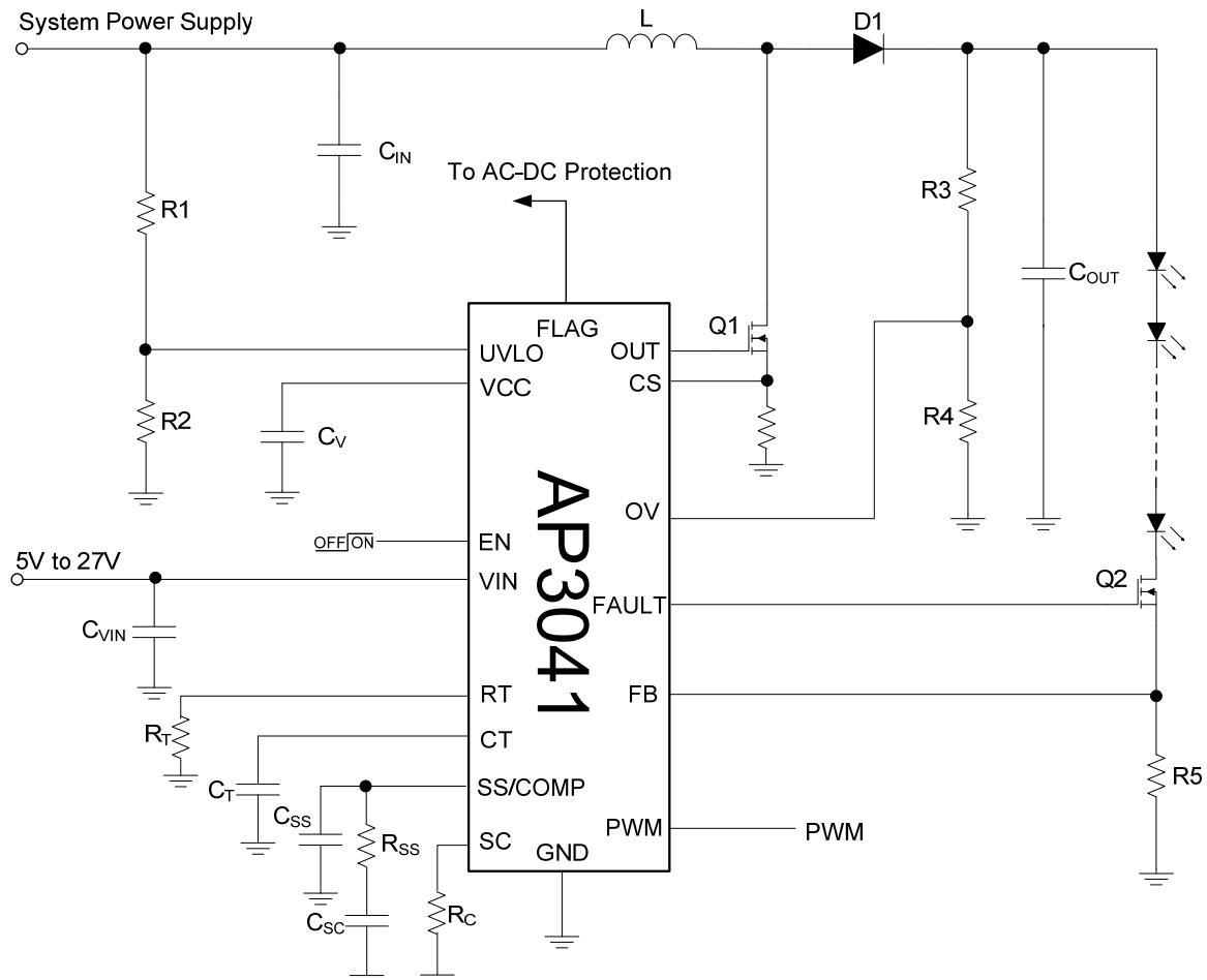
Figure 20. Typical Application Circuit of AP3041
