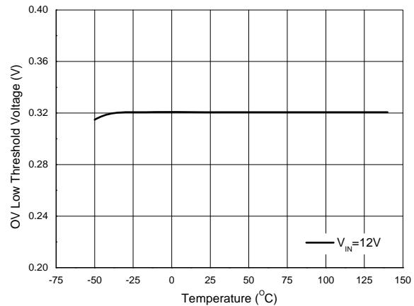
Figure 17. OV Low Threshold Voltage vs. Temperature
