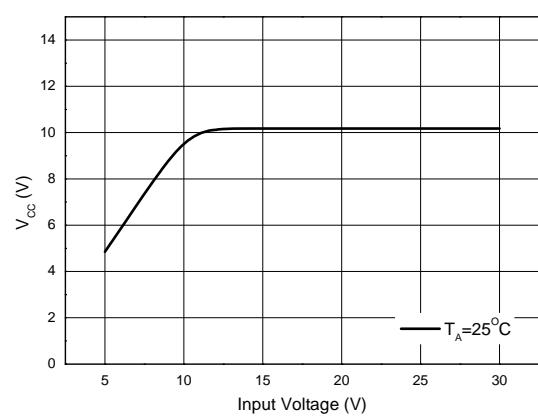
Figure 10.  $V_{CC}$  vs. Input Voltage
