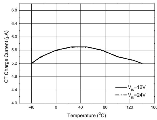
Figure 19. CT Charge Current vs. Temperature
