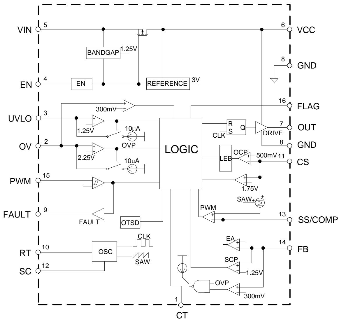
Figure 3. Functional Block Diagram of AP3041
