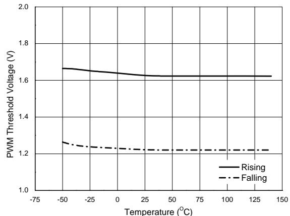
Figure 13. PWM Threshold Voltage vs. Temperature
