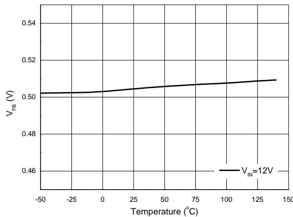
Figure 6.  $V_{FB}$  vs. Temperature
