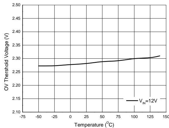
Figure 14. OV Threshold Voltage vs. Temperature
