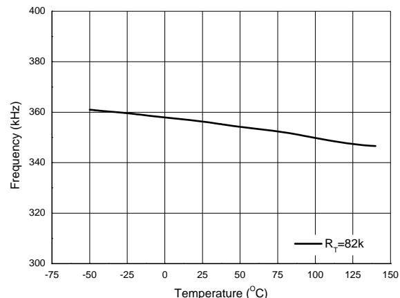
Figure 9. Frequency vs. Temperature
