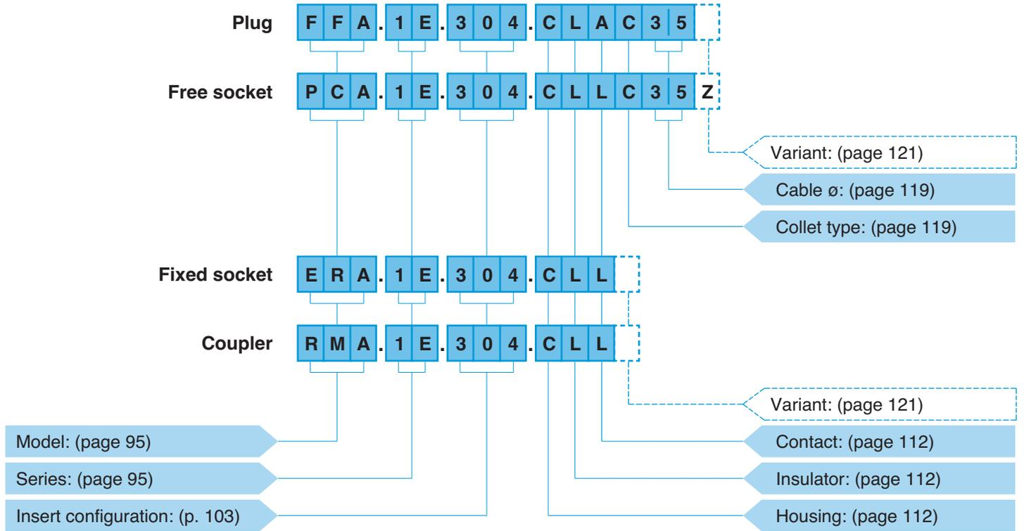
**FFA.1E.304.CLAC35** = straight plug with cable collet, 1E series, multipole type with 4 contacts, outer shell in chrome-plated brass, PEEK insulator, 2 male and 2 female solder contacts, C type collet for a 3.5 mm diameter cable.
