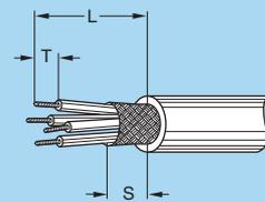
**Note:** 1) center wire L = 16.5. 2) center wire L = 20.5. 3) 5 center wires L = 20.5.
