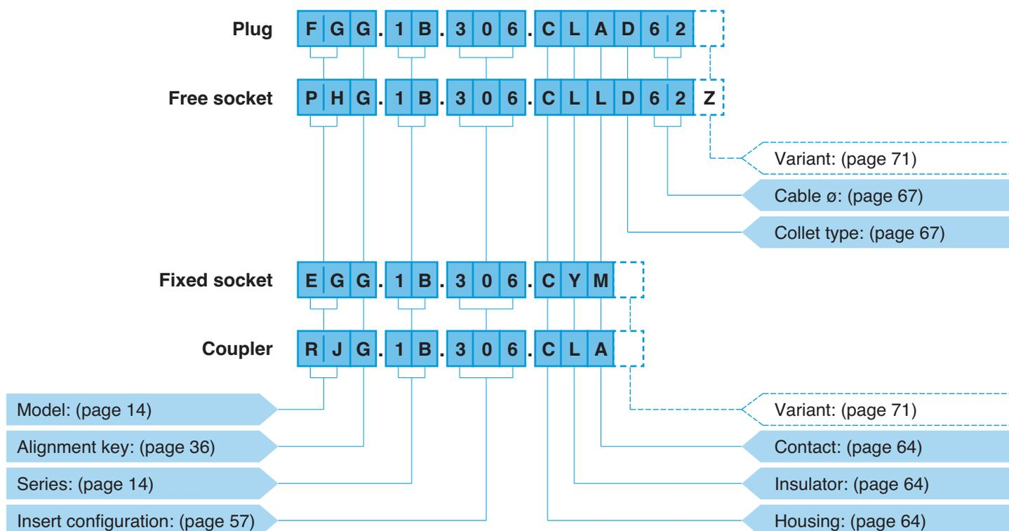
**FGG.1B.306.CLAD62** = straight plug with key (G) and cable collet, 1B series, multipole type with 6 contacts, outer shell in chrome-plated brass, PEEK insulator, male solder contacts, D type collet for 6.0 mm diameter cable.
