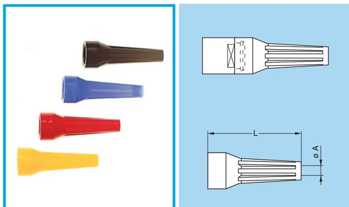
A bend relief made from thermoplastic polyurethane elastomer can be fitted over LEMO plugs and sockets that are supplied with nut for fitting such bend relief. They are available in nine different colours match with the GRA insulating washers (see page 149). Use the part numbers shown below to order this accessory separately.
