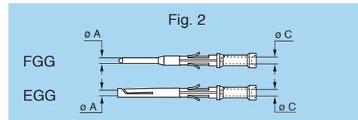
**Note:** a wide variation of strand number and diameter combinations are quoted as being AWG, some of which do not have a large enough cross section to guarantee a crimp as per either MIL-C-22520/1-01 or /7-01.
