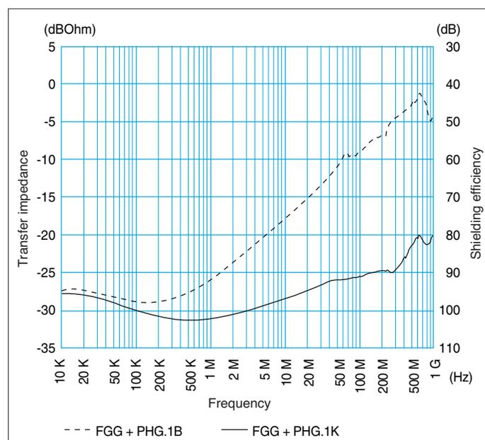
The performance of S and B series connectors is comparable to the results of measurements carried out on a pair of FGG + PHG.1B connectors.
