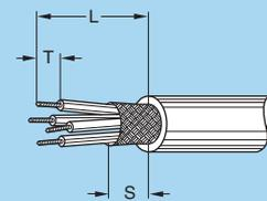
**Note:** <sup>1)</sup> In 0B and 1B series, «L» and «S» dimensions shall be increased by 2 mm for the largest collet (D56 in 0B series; D76 in 1B series). The tolerances on these dimensions are: L: ± 0.5 mm; S: ± 0.5 mm; T: ± 0.2 mm.
