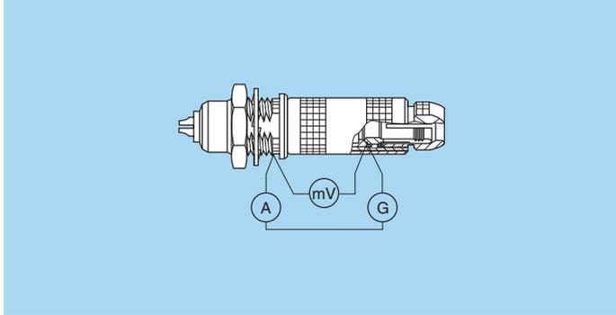
$R_1$  Values with earthing crown and latch sleeve or inner-sleeve nickel-plated.
