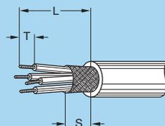
**Note:** the tolerances on these dim. are: L: ± 0.5 mm; S: ± 0.5 mm; T: ± 0.2 mm.
