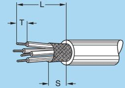
**Note:** 1) In 5B series, «L» and «S» dimensions shall be increased by 13 mm for the largest collet (D25).
