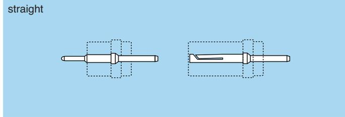
for wave soldering, we recommend removal the gold-plating from the contact end on the printed circuit side before soldering according to the assembly procedures.
