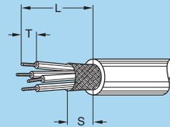
**Note:** <sup>1)</sup> crimp contacts are available only for connectors fitted with male contacts. The tolerances on these dim. are: L: ± 0.5 mm; S: ± 0.5 mm; T: ± 0.2 mm.
