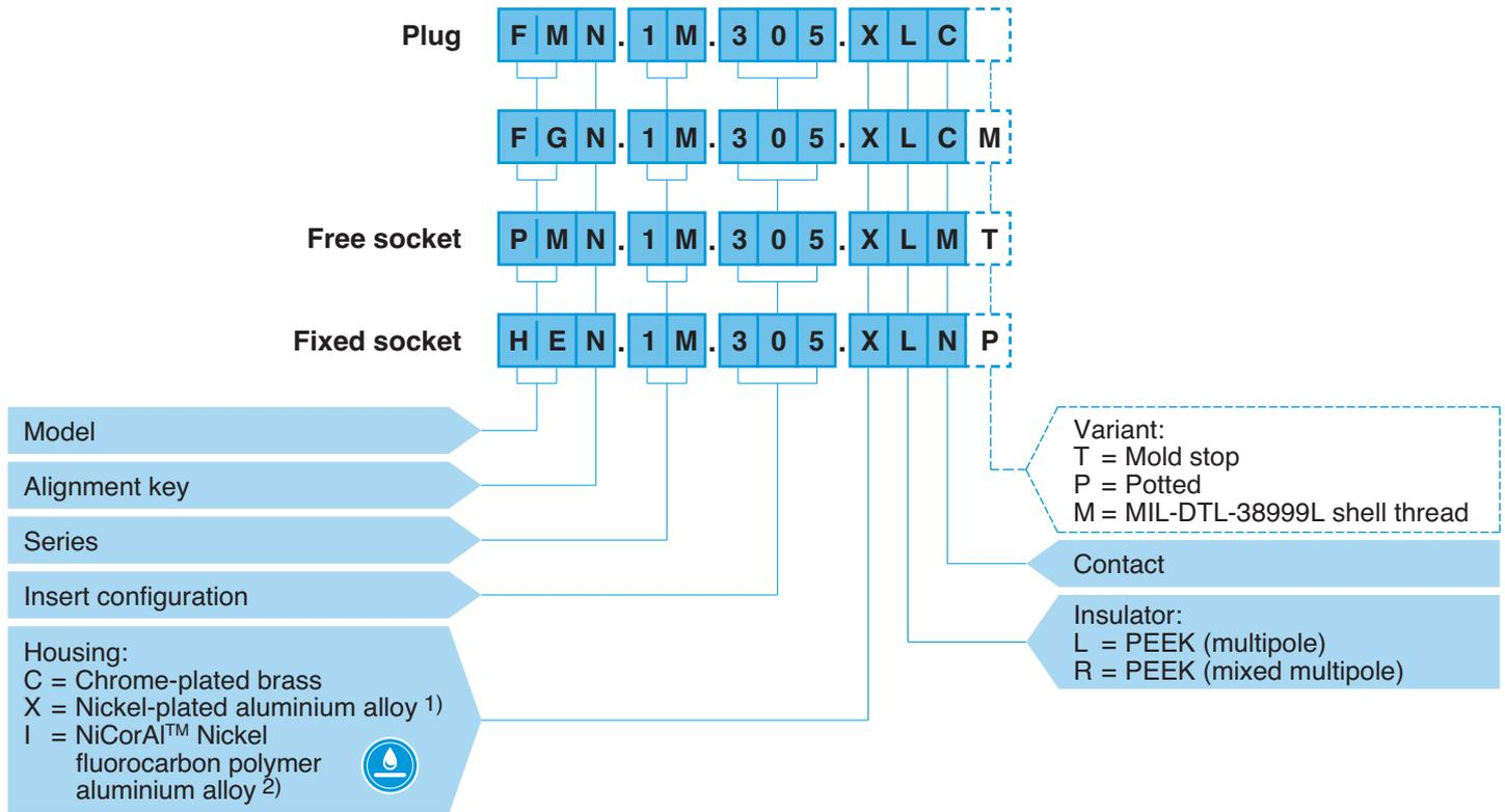
**FMN.1M.305.XLC** = straight plug with key (N), 1M series, multipole type with 5 contacts, outer shell in anthracite nickel-plated aluminium alloy, PEEK insulator, male crimp contacts
