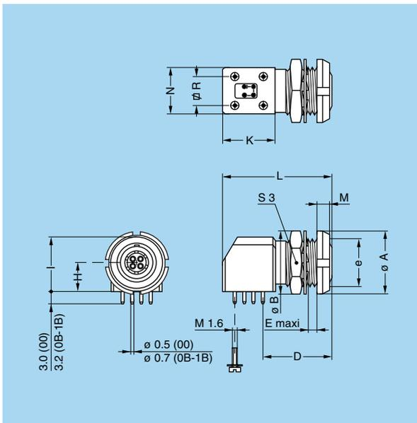
**Note:** In the 0B and 1B series, it is possible to replace the 4 ground pins by 4 screws (M1.6) add an «S» to the end of the part number. (e.g.: EXG.0B.307.HLNS).
