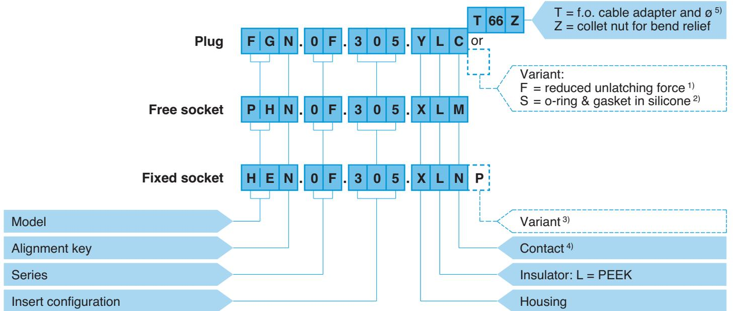
**FGN.0F.305.YLC** = straight plug with key (N), 0F series, multipole type with 5 contacts, outer shell in anthracite nickel-plated aluminium alloy, beryllium copper latch sleeve, PEEK insulator, male crimp contacts.
