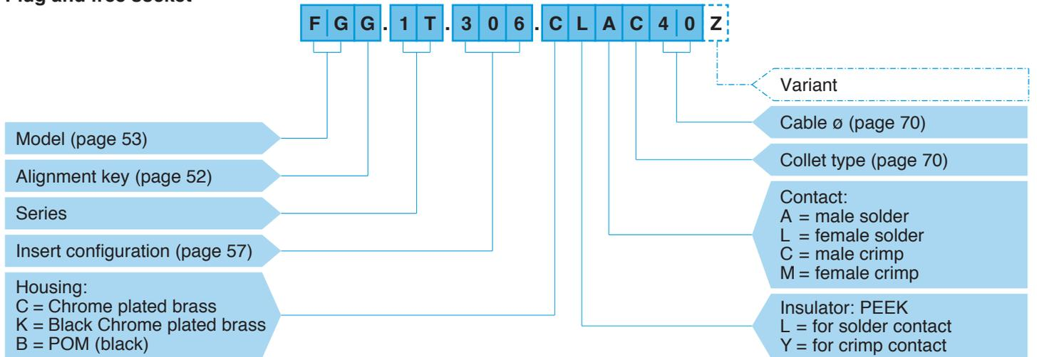
**FGG.1T.306.CLAC40Z** = Straight plug with key (G) and cable collet for bend relief, 1T series, multipole type with 6 contacts, outer shell in chrome-plated brass, PEEK insulator, male solder contacts, C type collet for 4.0 mm diameter cable and nut for fitting a bend relief.
