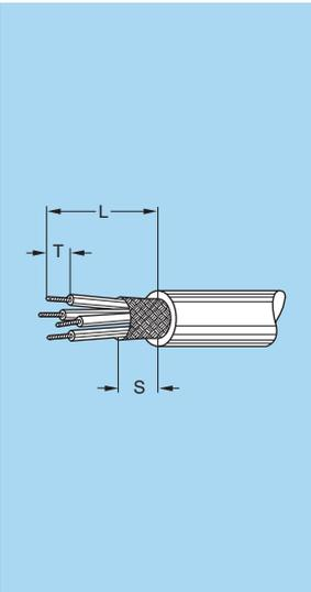
**Note:** <sup>1)</sup> In 1B series, «L» and «S» dimensions shall be increased by 2 mm for the largest collet (D76 in 1B series).
