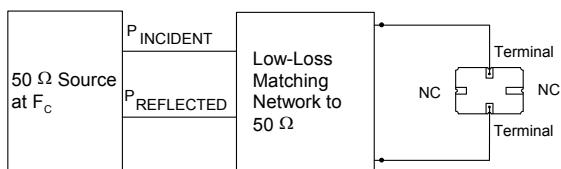
$$\text{CW RF Power Dissipation} = P_{\text{INCIDENT}} - P_{\text{REFLECTED}}$$
