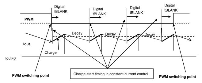
The digital tBLANK time is inserted immediately after the switching timing of externally applied PWM signals (CLK\_X and ENABLE\_X) such as the switching timing between short brake and charging, and also when the charging in constant-current chopper drive is started.
