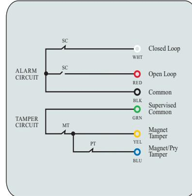
Dual alarm contacts both closed loop, with tamper circuit, closed loop.
