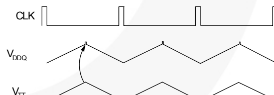
Figure 9. Noise-Susceptible In-Phase Operation for DDR2
