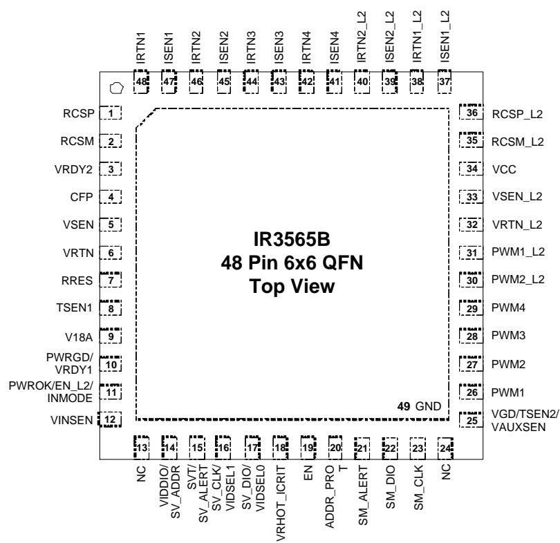
Figure 1: IR3565B Pin Diagram Enlarged
