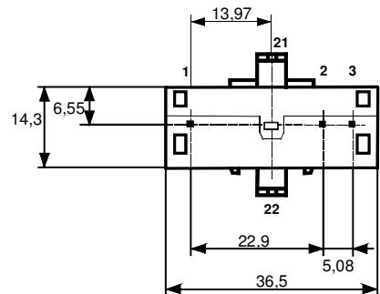
Tolerances grid distance  $\pm 0.2\text{mm}$
