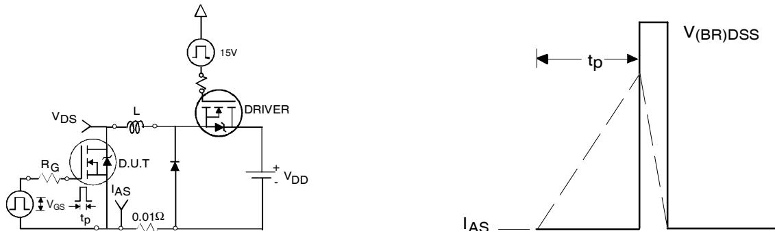
**Fig 24a.** Unclamped Inductive Test Circuit
