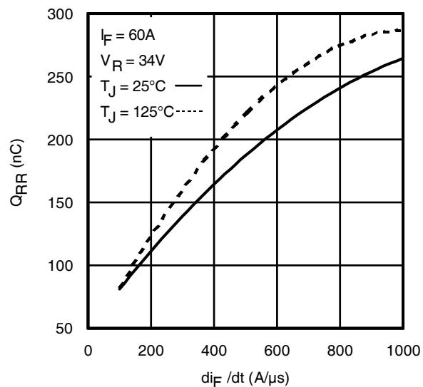
**Fig. 19** - Typical Stored Charge vs.  $di_F/dt$
