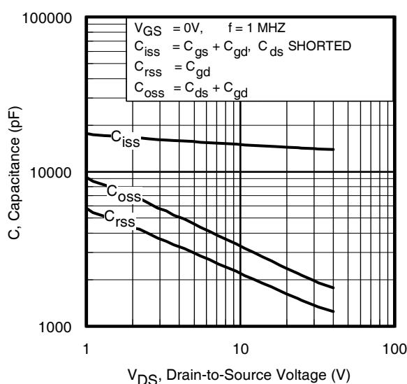
**Fig 5.** Typical Capacitance vs. Drain-to-Source Voltage
