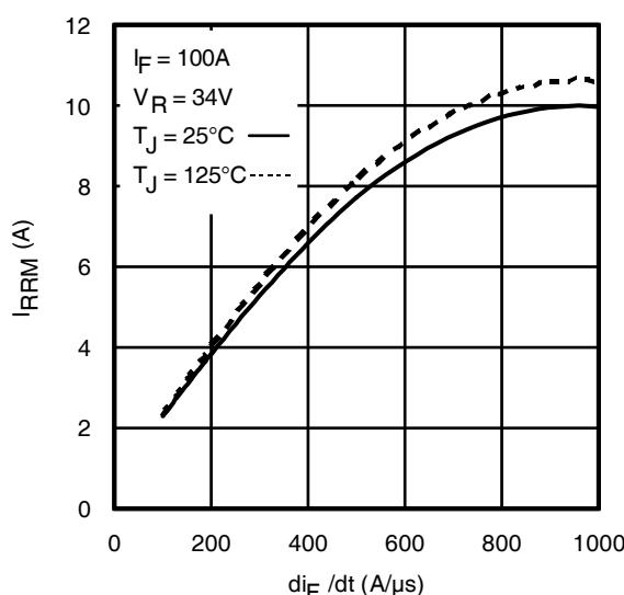
**Fig. 20** - Typical Recovery Current vs.  $di_F/dt$
