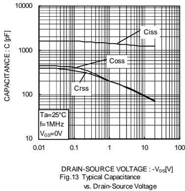
Fig.13 Typical Capacitance vs. Drain-Source Voltage
