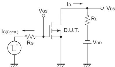
Fig.4-1 Gate charge measurement circuit
