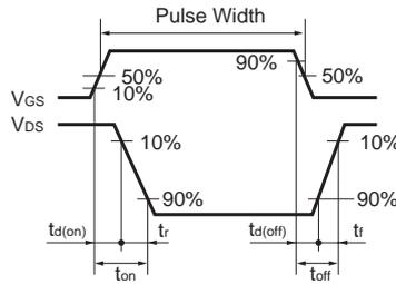
Fig.1-2 Switching Waveforms
