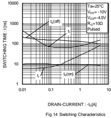
Fig.14 Switching Characteristics
