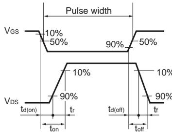
Fig.3-2 Switching waveforms
