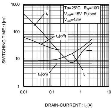
Fig.13 Switching Characteristics
