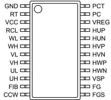
Figure 3. Pin configuration
