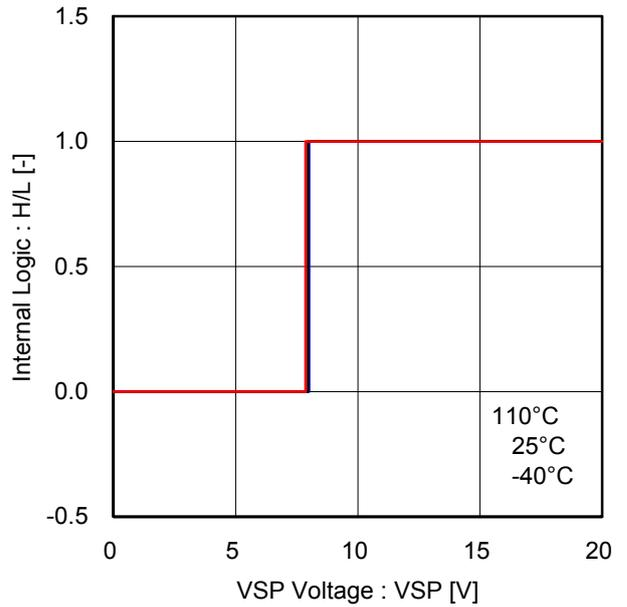
Figure 18. Testing mode threshold voltage
