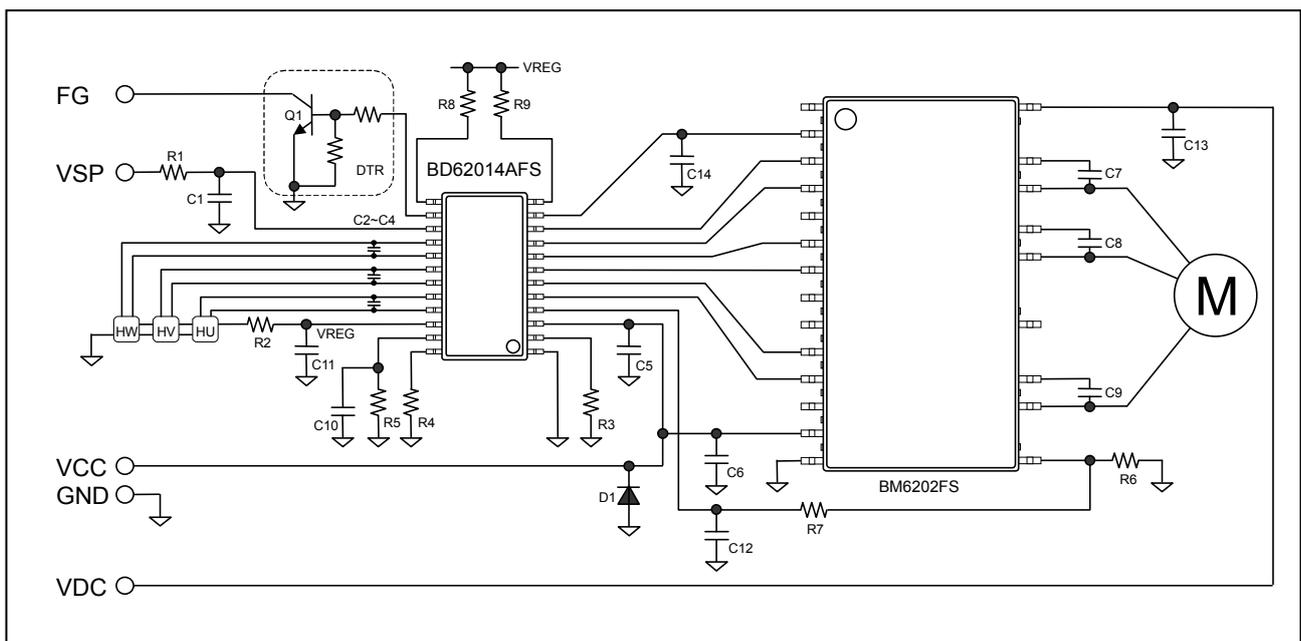
Figure 1. Application circuit example - BD62014AFS & BM6202FS
