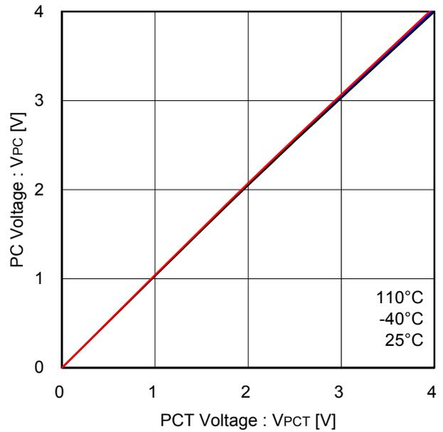
Figure 30. PCT - PC linearity
