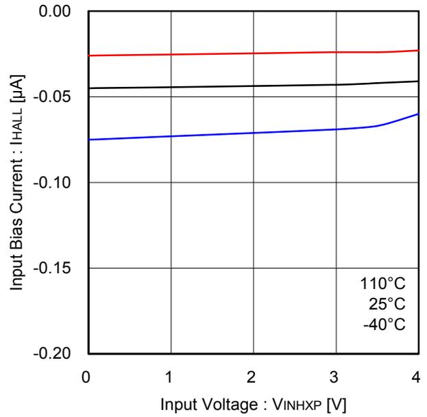
Figure 14. Hall comparator input bias current (HXP, HXN)
