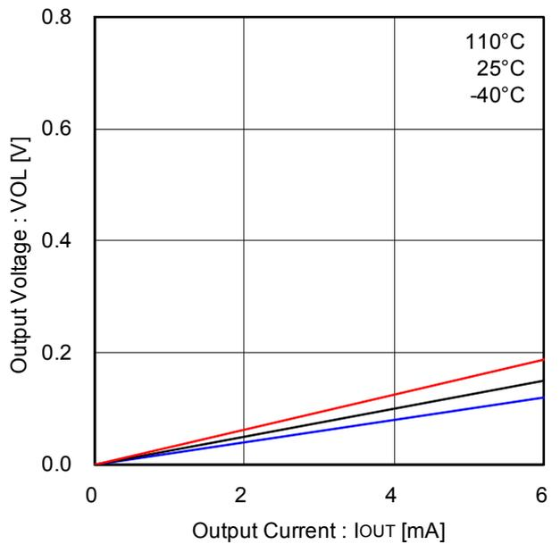
Figure 20. Low side output voltage (FG)
