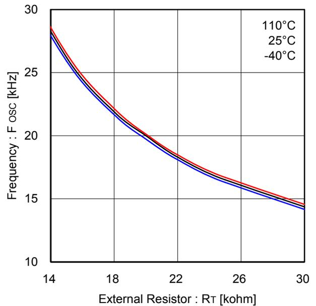
Figure 32. Carrier frequency -  $R_T$
