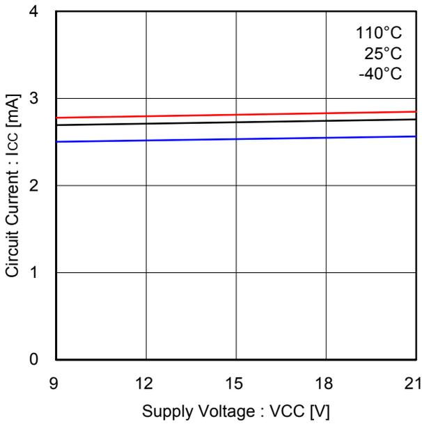
Figure 9. Circuit current
