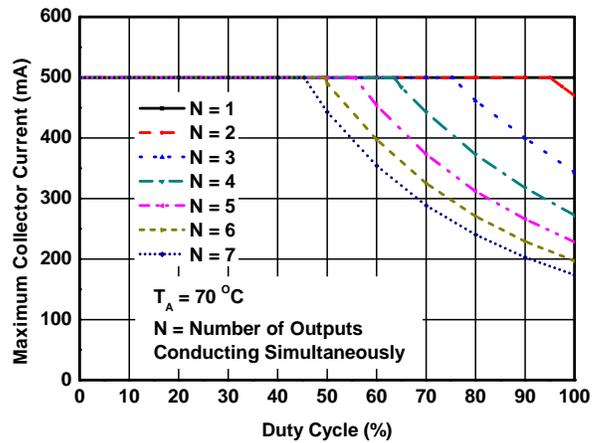
Figure 14 Maximum Collector Current vs. Duty Cycle
