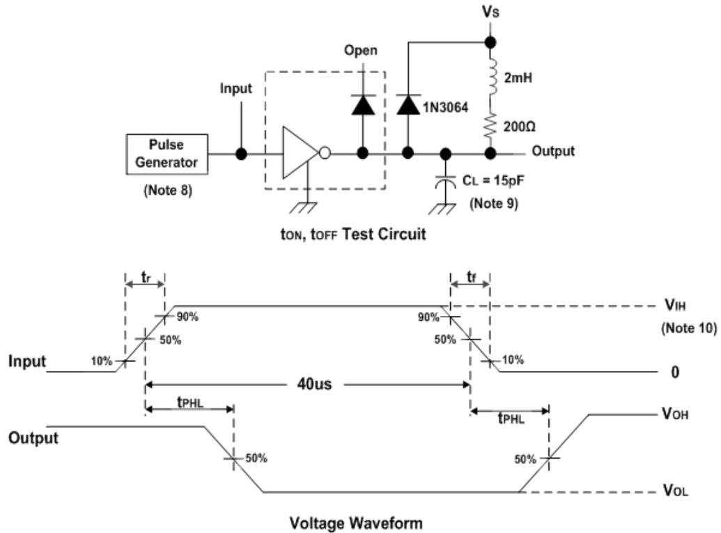
**Fig. 10 Latch-Up Test Circuit and Voltage Waveform**
