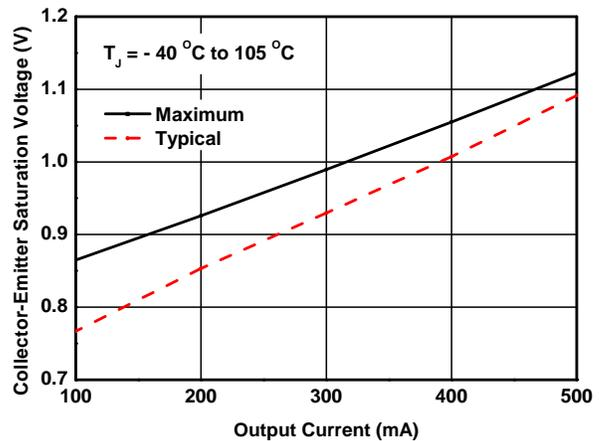
Figure 16. Collector-Emitter Saturation Voltage vs. Output Current
