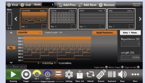
Digital Pattern Generation (DPG functionality)
