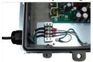
6) Using waterproof outdoor rated Cat5e Ethernet cable, thread through cable glands or conduit piping to the appropriate RJ45 connector and ensure each portal is properly sealed.
