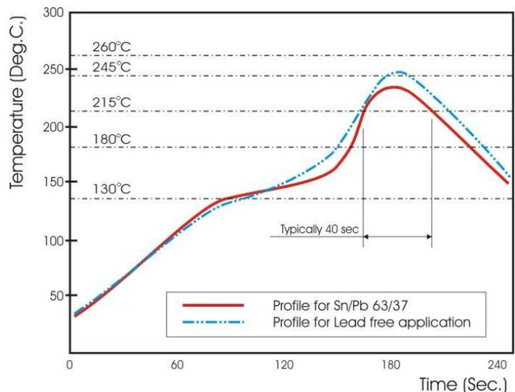
Fig 3. Infrared soldering profile for Chip Resistors WW18X
