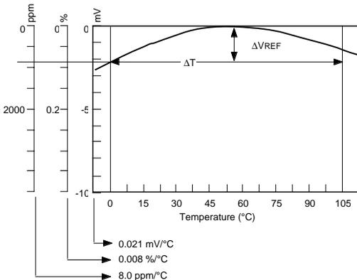
$$\bullet \text{ TC in mV}/^\circ\text{C} = \frac{\Delta V_{REF}}{\Delta T_A} \quad (\text{mV})$$
