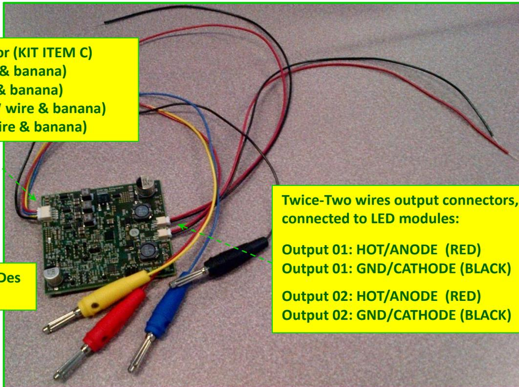
Four wires input connector (KIT ITEM C)
