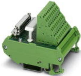
VARIOFACE module, with spring-cage connection and D-Subminiature socket strip, for mounting on NS 35/7.5 or NS 32, 25-pos.
