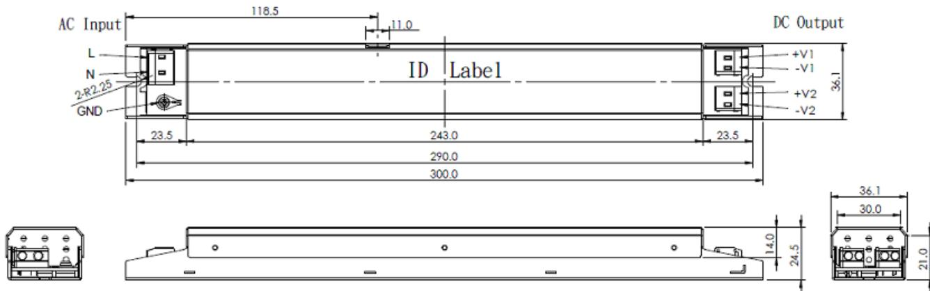
Input Connector: WAGO 235-502 2Pin or Equivalent
