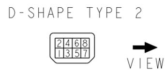
1. APPLICABLE CABLE: RECOMMENDED AWG30~26 X 8C
