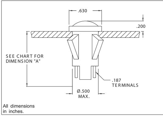
Mounting: Will snap-fit into Ø.500/.505 hole in panels .020/.100 thick. Push-on speednut SN0461 also available.
