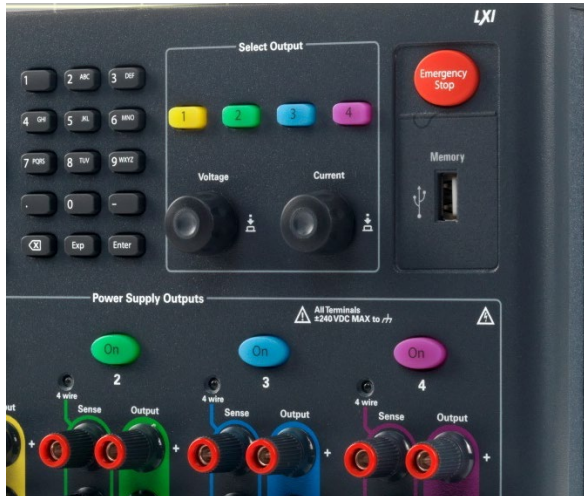
Figure 11. The N6705's front panel USB port.
