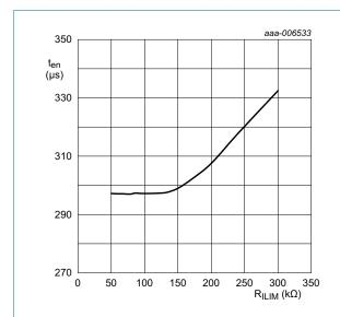
EN = 1.5 V; VINT = 4 V; R<sub>L</sub> = 150  $\Omega$ ; C<sub>L</sub> = 100  $\mu$ F; T<sub>amb</sub> = 25 °C.
