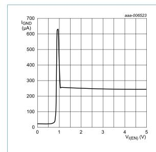
Fig 8. Typical ground current versus input voltage
