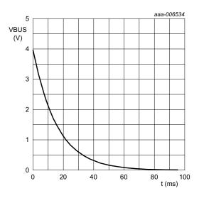
EN = 1.5 V; VINT = 4 V; R<sub>L</sub> = 150  $\Omega$ ; C<sub>L</sub> = 100  $\mu$ F; R<sub>ILIM</sub> = 50 k $\Omega$ ; T<sub>amb</sub> = 25 °C.
