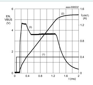
EN = 1.5 V; VINT = 5.5 V; R<sub>L</sub> = 150  $\Omega$ ; C<sub>L</sub> =220  $\mu$ F; R<sub>ILIM</sub> = 50 k $\Omega$ ; T<sub>amb</sub> = 25 °C.
