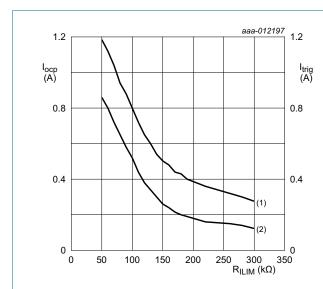
$V_{I(VINT)} = 5 \text{ V}; T_{amb} = 25 \text{ }^{\circ}\text{C}.$
