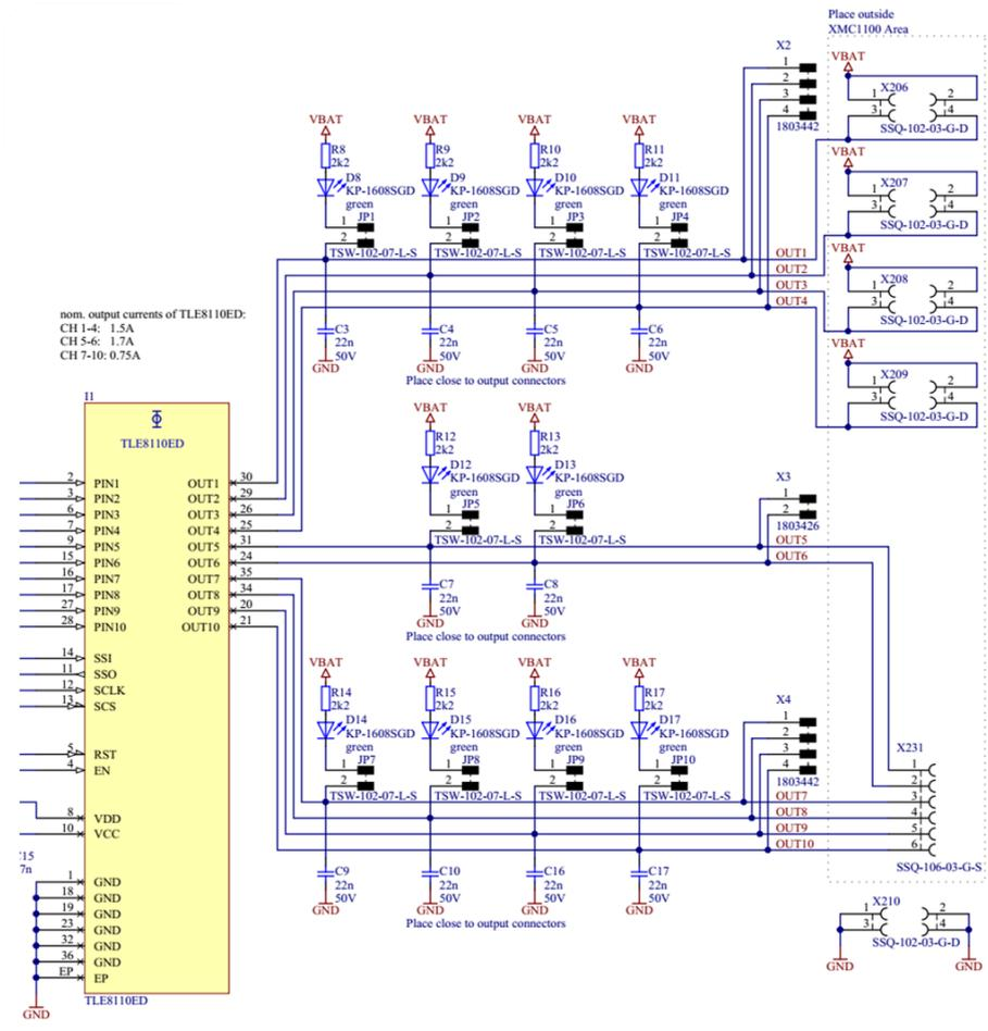
**Figure 1-8 Load connection and indication LED circuit**
