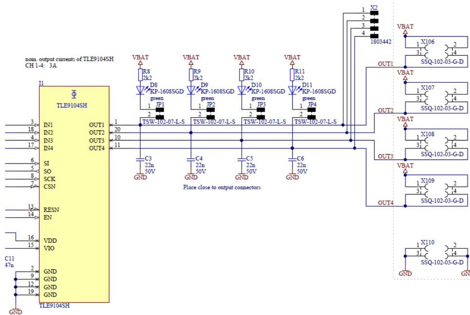
**Figure 1-4 Load Connection and indication LED circuit**
