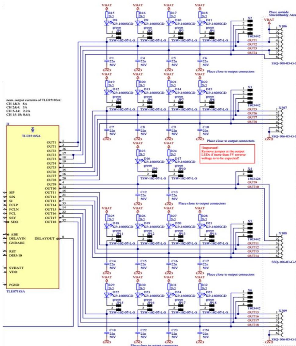
**Figure 1-12 Load Connection and indication LED circuit**
