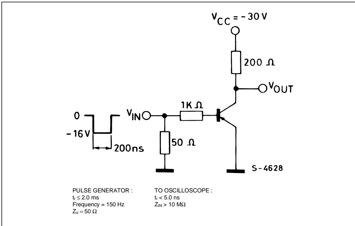
Test Circuit for  $t_{off}$ ,  $t_o$ ,  $t_f$ .
