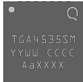
28 lead 5x5mm QFN package
