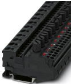
Fuse terminal block for cartridge fuse insert, cross section: 0.5-10 mm², AWG: 20-8, width: 12.2 mm, color: Black
